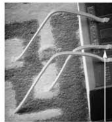
Loop starts at the die since there is no ball
