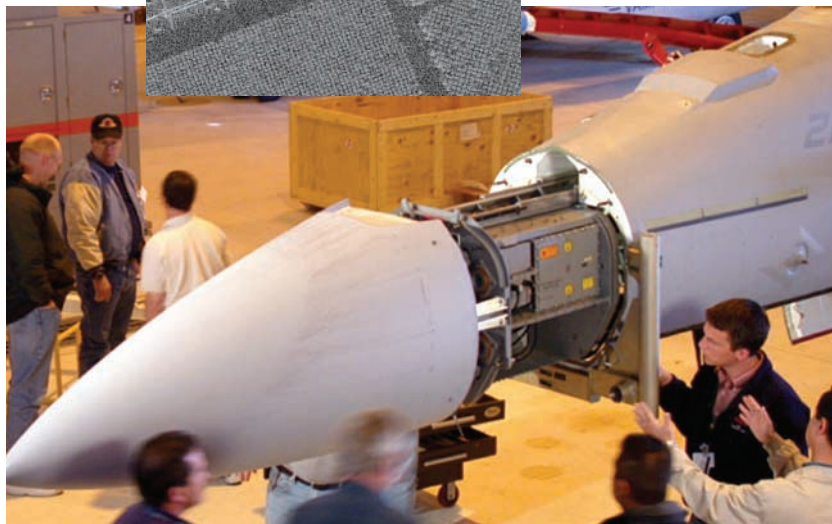
Below, the first APG-79 radar installed at China Lake last year. Left, one of the first declassified SAR maps, showing orange groves, an access road, and livestock pens.
